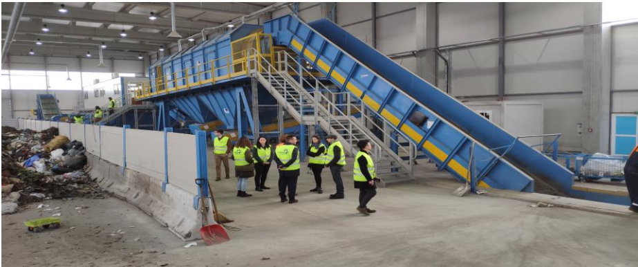
Figure 3. Technological line of secondary selection - MRF (Material Recovery Facility)
