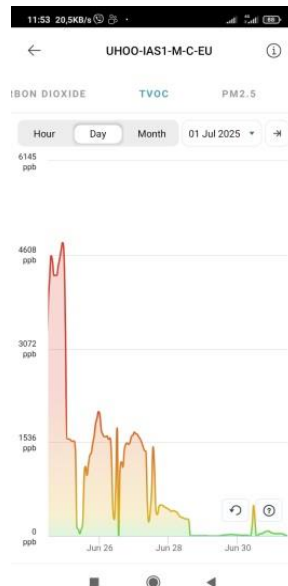
Figure 2. TVOC oscillations during few days in June. TVOC increases as the occupants enter the office and then gradually decrease after their leave.
